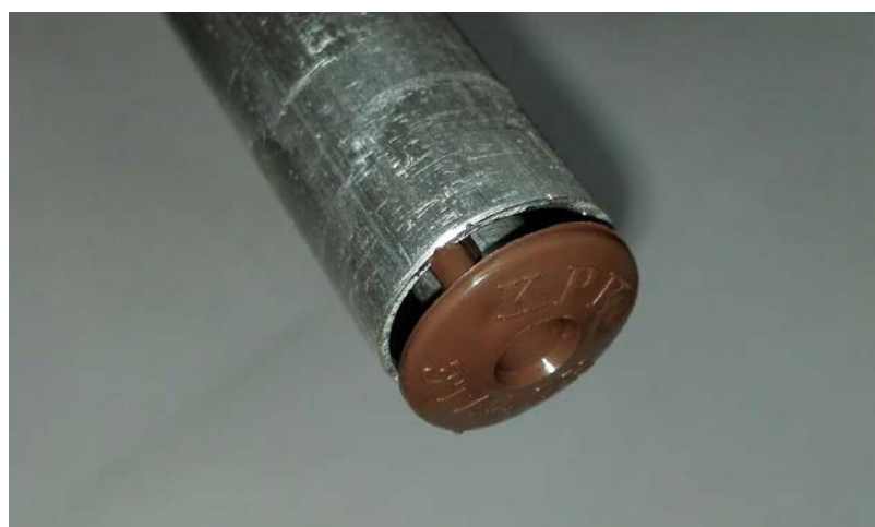
Figure 3 – Sensor blind plug
